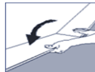
Fig 1. First plank, first row. Place a spacer of 12-15 mm thickness to the left and position the plank against the wall. Later, after 3 rows, you can easily position the flooring against the front wall with distances 12-15 mm.
