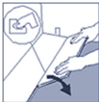
Fig 3. Tilt angle the panel down. During the angle process make sure the panels are tight against each other. Afterwards press down or slightly tap down at the short end or long edge of the installed plank till its flat. No major force is required.
