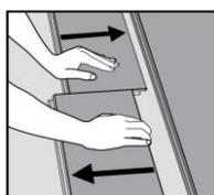
**Disassembling (without tool).** Your floor can very easy be disassembled, which enables replacement during installation and also during use. **Fig 11.** Separate the whole row by carefully lifting up and slightly knocking just above the joint. Fold up and release the whole long side. **Fig 12.** Disassemble the panels by sliding horizontally. (Do not fold up!)
