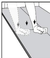
**Figs 8c** As it flattens itself to the floor press or gently tap the top of the short end of the installed panel until it clicks. Finish installing this plank by tapping it with a tapping block on the long side to ensure secure installation.
