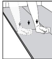
**Figs 8c** As it flattens itself to the floor press or gently tap the top of the short end of the installed panel until its flat. Finish installing this plank by tapping it with a tapping block on the long side to ensure secure installation.
