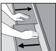
**Disassembling** Your floor can be disassembled, which enables replacement during installation and also during use. Separate the whole row by carefully lifting up and slightly knocking just above the joint. Fold up or angle and release the whole long side. Disassemble the planks by sliding horizontally where possible or fold up and angle to release.
