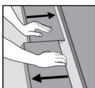
Disassembling (without tool). Your floor can quite easy be disassembled, which enables replacement during installation and also during use. Fig 11. Separate the whole row by carefully lifting and slightly knocking just above the joint. Fold up and release the whole long side. Fig 12. Disassemble the panels by sliding horizontally. (Do not fold up!)
