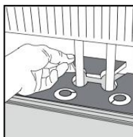
Radiator pipes, installation at radiators. Drill the holes 20 mm larger than the diameter of the pipes. Cut out the panel (with the thinnest blade possible) as per diagram. Install the plank as per normal. Glue the cut-out piece back again.
